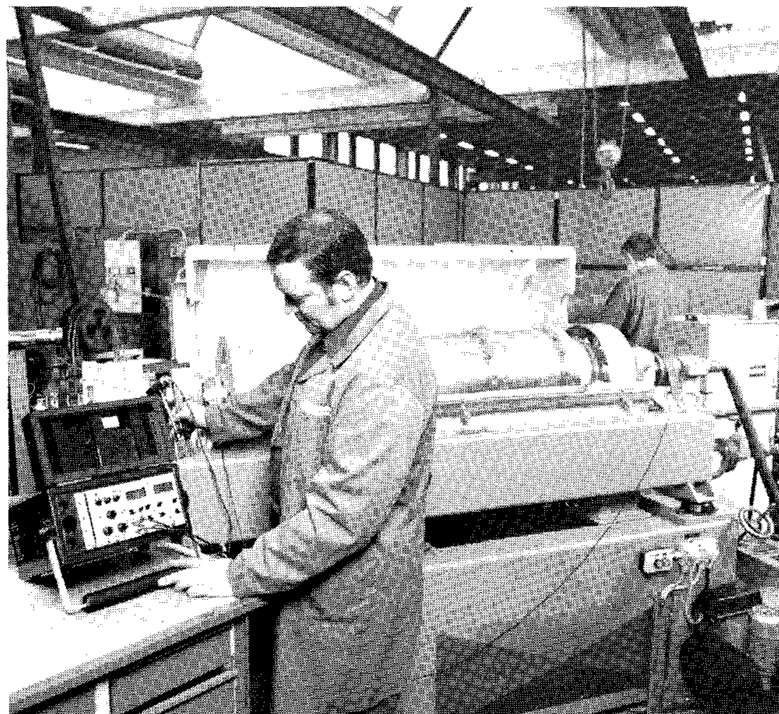
Fig. 24. To the left, the Balancing Set Type 3537. To the right, balancing a Alfa-Laval NX 418 decanter centrifuge
